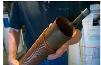
**Drain water heat recovery unit**
